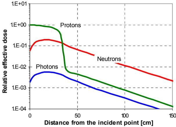
Fig. 5. Attenuation of the effective dose in heavy concrete for parallel beams of 500 MeV protons. The different curves represent the separate contributions to the effective dose from protons, neutrons and photons.
