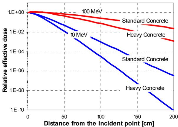
Fig. 4. Relative effective dose as a function of distance from the incident point, in standard and heavy concrete for parallel beams of 10 MeV and 100 MeV neutrons. The effective dose includes the contributions from all secondary particles, i.e. the neutrons, photons and protons that are created when the incident high-energy neutrons are moderated.
